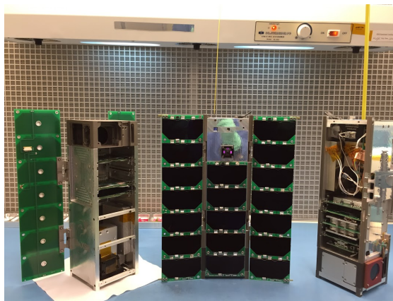
Figure 2: Iterations of the MinXSS CubeSat from left to right: a prototype model used for early testing, Flight Model 1 which deployed from the ISS in 2016, and Flight Model 2 that will launch in 2018 [9].
